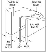
Panel assembly cross section. Panel assembly rear view.
